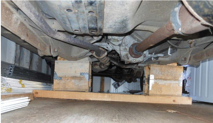
Wooden blocks under the front axle of the car
